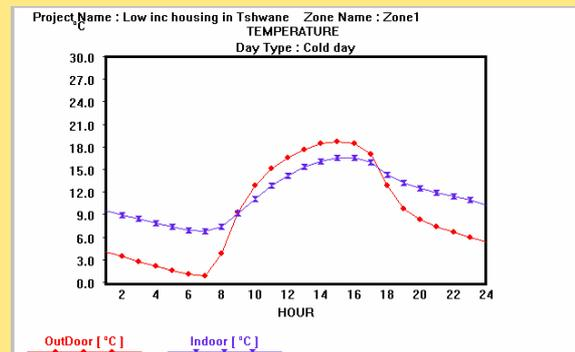
The graphs show indoor and outdoor temperatures for a low income house in Gauteng – without passive solar design features (below), and considering key passive solar interventions such as proper orientation, window shading, roof insulation and wall materials (above). The temperature extremes experienced by the former are excessive, and are greatly reduced in the house where such intelligent design is considered.
