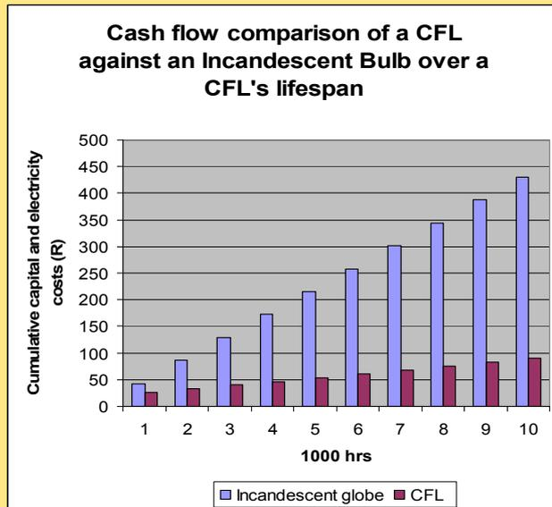
This graph compares the cost of purchasing and using a CFL with the cost of purchasing and using an incandescent bulb over the same time frame. In this case an 18W CFL (costing R18 with a lifespan of 10 000 hrs) is compared with a 100W incandescent bulb (costing R30 with a lifespan of 1000 hrs).
